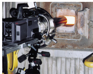
Special high temperature vortex tubes keep a borscope lens cool while inserted into a 1200°F (650°C) boiler porthole.
